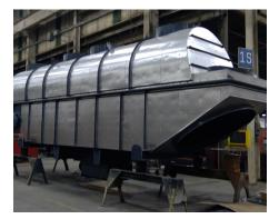
Wet Feed Capacity: 20 TPH Wet Feed Moisture: 22% Product Discharge Moisture: 11.5% Pellet Size: 5/16" Ø x 1/2" long Drying Air Temperature: 400F Maximum Cooling Air Temperature: Ambient
